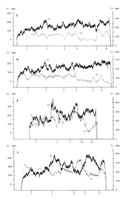
Fig. 16. Continuous scanning profiles for Ti- and Cr- $K\alpha$  radiation across the corundum RGM 107 199.
