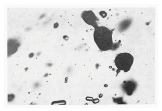
Fig. 14. Pyrrhotite and apatite crystals in almandine garnet RGM 163 158, 40x.
