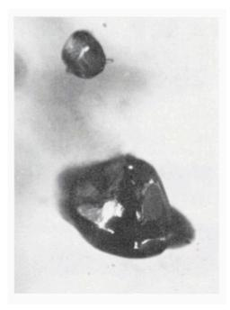
Fig. 15. Pyrrhotite crystals in almandine garnet RGM 163 158, 90x, both reflected and transmitted light.
