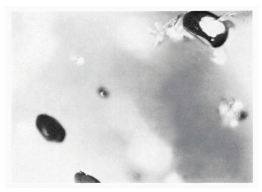
Fig. 4. Rutile crystals in rhodolite garnet RGM 163 171, 65x, reflected light.
