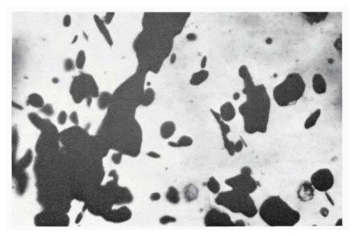
Fig. 22. Graphite flakes in deep violet corundum RGM 163 153, 60x.
