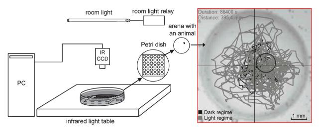
*Fig. 1.* Schematic representation of a video tracking system for the automated analysis of animal movement behaviour. The right part of the figure shows an example trajectory of an individual of *M. tardigradum* over the first 24-hour period. The circle indicates the last position of the animal (see embedded supplementary video).
