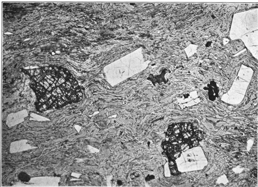
Vitrophyre. Well developed fluxion structure. Phenocrysts of plagioclase and partly altered olivine. Ordinary light. 50 X.
