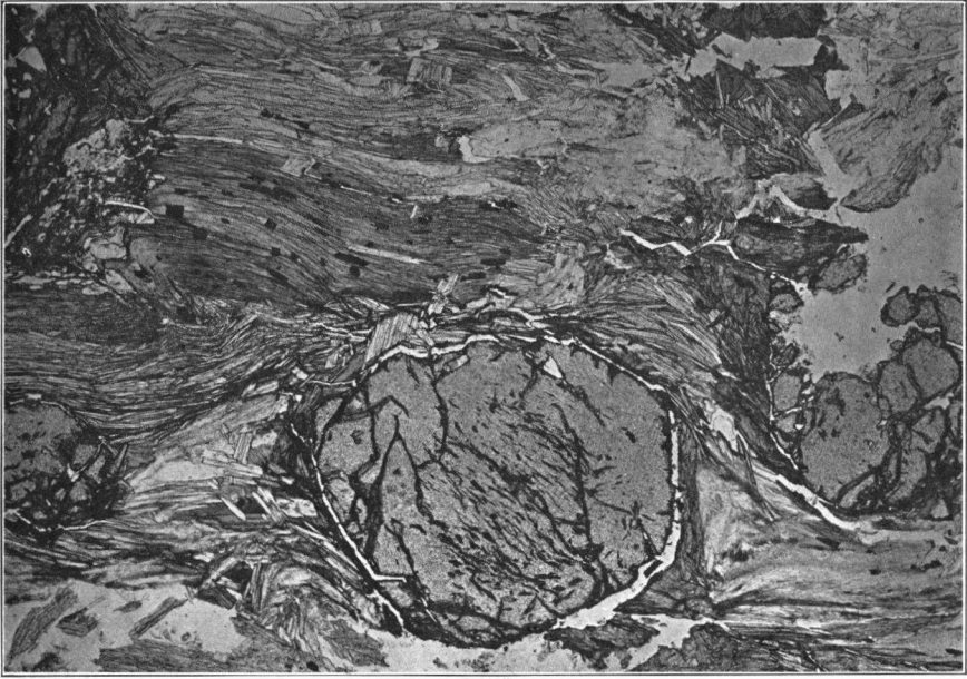
Meso-Garnet-Muscovite-gneiss. Garnet with inner relict structure. Recrystallization of muscovite visible in the upper half of the photograph. Ordinary light. 25 \times .
