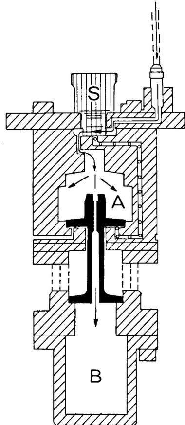
Fig. 3. Pneumatic sound source.
