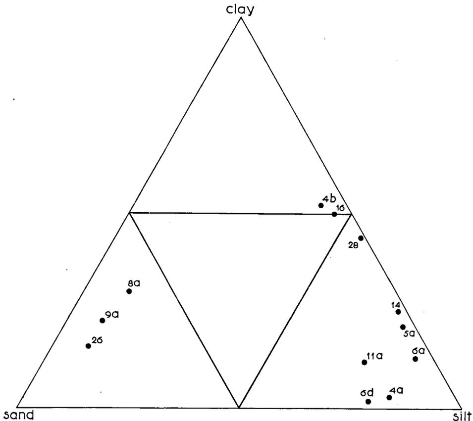
Fig. 5. Sand-silt-clay triangle-diagram of the fine-grained sediments.
