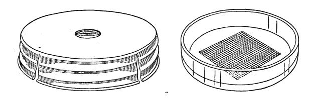
The second improvement is the etching of a net of sq. millimetres in the glass bottom of petri dishes, at least in most of the central portion of these. This facilitates taking exact measurements under water; no loose special metal or glass millimeter strips are needed any longer. The etching proved to be rather expensive in Holland; each dish costed about US \$.4.-, but we are very glad to have them.
